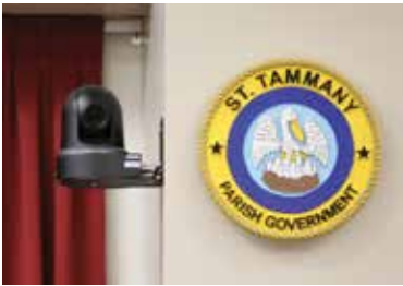
Access St. Tammany has installed three JVC KY-PZ100 PTZ cameras to improve its coverage of government meetings in the St. Tammany Parish Council chambers.
