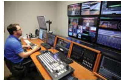
By using a JVC RM-LP100 remote camera control and three JVC KY-PZ100 PTZ cameras to cover meetings for the St. Tammany Parish Council and other departments, Access St. Tammany is significantly reducing personnel costs.
