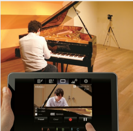
The camera on the stage can be remote controlled from a smart device. Controls include REC/STOP, Zoom, Focus, Iris and more detailed settings while viewing live images from the smart device screen.
