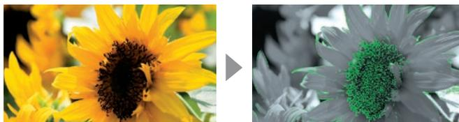
When the Focus Assist function is set to ON, objects that are in focus appear with colored edges (selectable from red, green or blue) as seen here.
