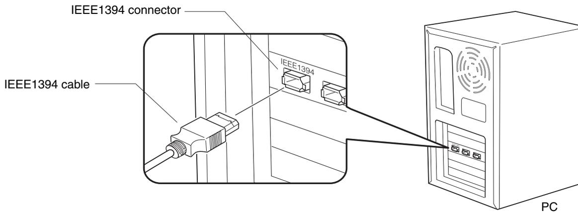
When connecting the IEEE1394 cable from camera recorder to other IEEE1394 device such as PC, make sure the following instructions, otherwise the IEEE1394 circuit device may be destroyed.
