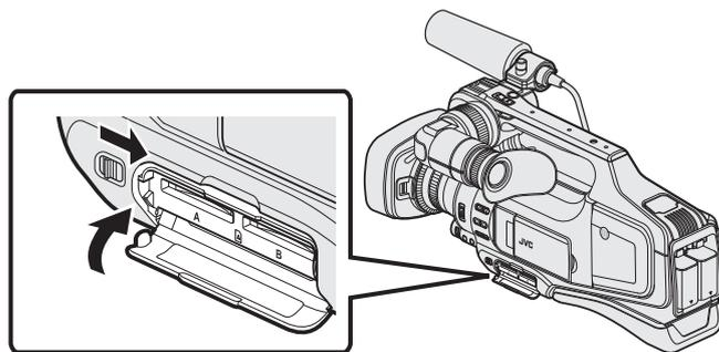
• After closing the door, slide the “DOOR LOCK” lever to the right to lock the door.
