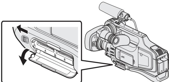
• Slide the “DOOR LOCK” lever to the left, and pull the door towards you.
