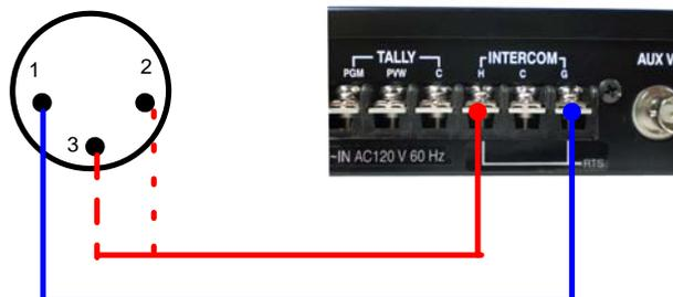
When connecting to a 2 wire Clear-Com audio system, wire the Clear-Com three pin microphone XLRs to the RM-HP250AU as shown below.
