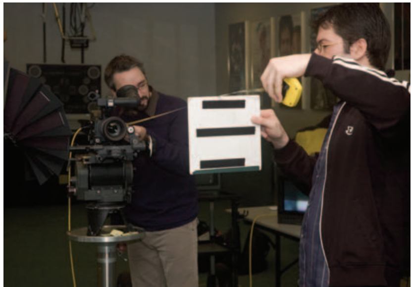
Adjusting the backfocus
