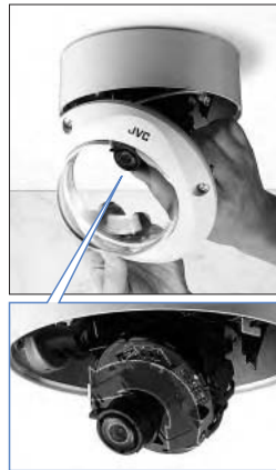
5. Adjust the angle and focus testing with the dome cover.
