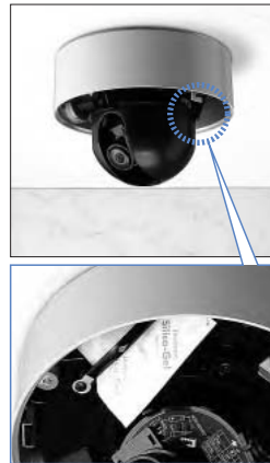
6. After lens setup, install silica gel bag and fit the inner cover.
