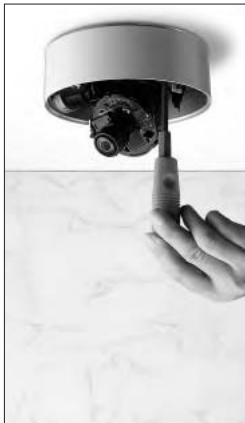
4. Using a screwdriver secure the camera unit to the base by tightening the 2 screws.
