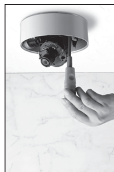
4. Using a screwdriver secure the camera unit to the base by tightening the 2 screws.
