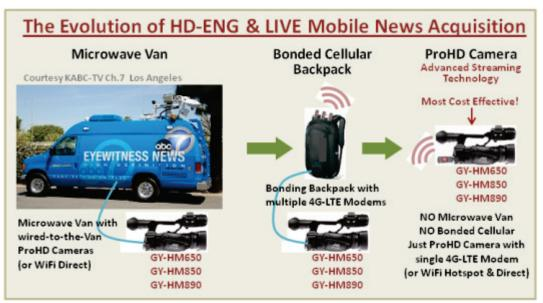
The above illustration shows the "evolution" of LIVE Mobile News Acquisition and Backhaul over the past five years, from the Microwave Van through the Bonding Backpacks to the "lone ranger" video journalist (VJ) with just the 4G-LTE USB Modem-fitted ProHD Camera (switchable to WiFi Hotspot/Direct operation). It is obvious which is the most cost-effective.
