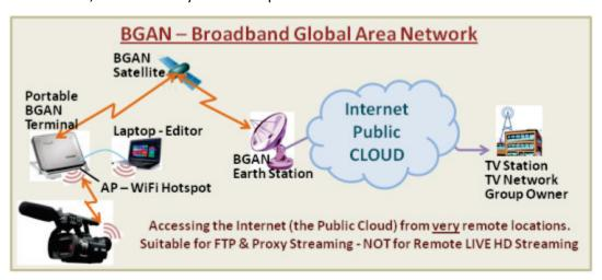
The portable BGAN terminal (the size of a larger laptop, including satellite transceiver/antenna) is self-contained, only at the mercy of a power source, being mains plug-in or battery.
