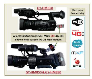
Illustration shows the built-in capabilities of the cameras: WiFi USB Modem or 4G-LTE USB Modem may be plugged into the cameras' full size USB Host port to provide wireless connectivity to the Internet.
