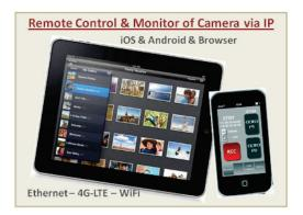
can download (push) Metadata to the Camera, to be embedded in clips as specified. The remote control connection may also monitor the LIVE shoot or play back clips stored on SD memory cards by selecting from thumbnails.
