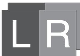
Shrinks the size of the left and right images by half and displays them side by side. The format is compatible with most recent 3D-compatible displays. This format is very convenient because of its high compatibility with existing recording and transmission systems though the horizontal resolution is reduced to half.
