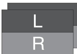
Shrinks the left and right images by half vertically and displays them top and bottom. The vertical resolution is reduced to half but the horizontal resolution is free from degradation if you use a monitor with polarized filter system.
