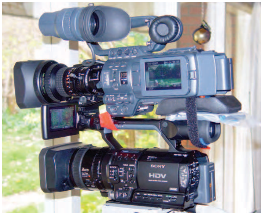
above: In a side-by-side test (actually top and bottom), wide-angle lockdowns of shaded foliage moving in a gentle breeze showed smooth motion in Sony's recording, whereas blocks of leaves in HD100's pictures tended to sit in place for a few frames and then jump slightly to their new positions (as the jumps tended to happen synchronously, several times a second, I'm guessing that they mostly jumped on I-frames).
