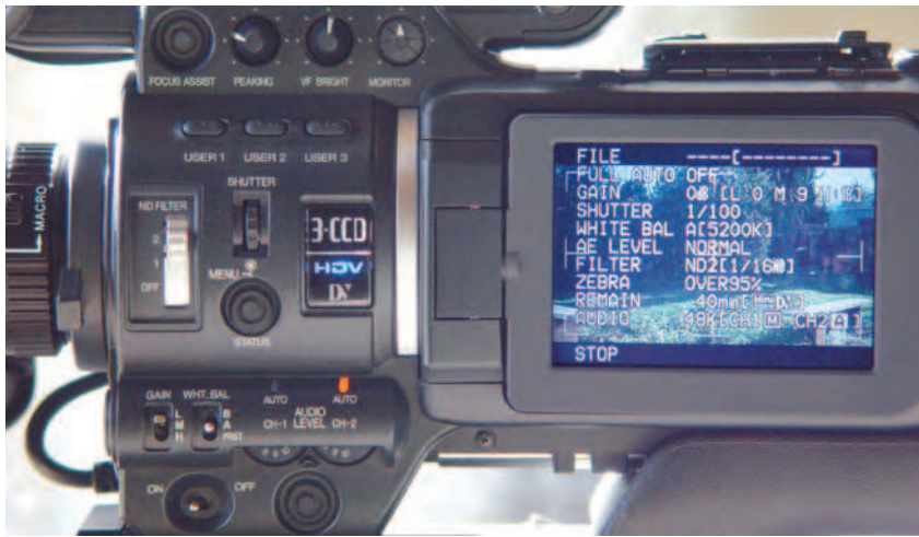
above: There's a slide switch for the built-in ND filter, providing two and four stops of attenuation. A thumbwheel offers shutter speed selection, and a push button cycles through operational and status displays (including, thankfully, an uncluttered display) or, with a longer push, brings up the camera's extensive and well-organized menus. Three user buttons allow some control customization and can be used to navigate the menus if you prefer not to use the shutter wheel. Format lamps show whether HDV or DV is being recorded.
