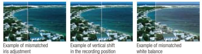
• **Horizontal (R) Shift:** In order to check vertical shift or color discrepancy, the right camera image can be shifted to the left to overlap with the left camera image, which is static.
