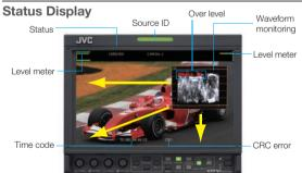
\*Choose from four positions to display the waveform monitoring. \*The level meter can also be displayed vertically.
