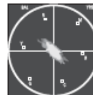
Difference Vectorscope: Displays the differential between the two signals in vectorscope.
