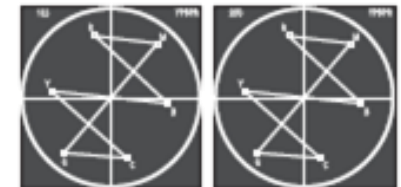
Parallel Vectorscope: Displays the two signal scopes side by side.
