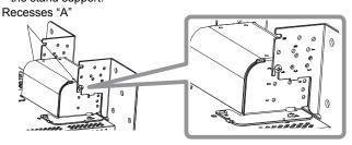
4 Adjust the position so that the screw holes on the stand support align with right and left screw holes "C" and "E" on the bottom plate, tighten the two stand screws on one side (four screws on both sides), and finally retighten the temporarily set screws to lock the stand support and the bottom plate.
