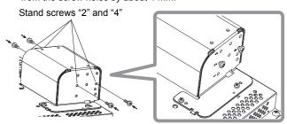
3 Tighten commercially available screws in the 6 holes shown in the figure below to install the monitor on the wall.
