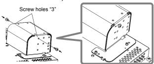
**3** Hook right and left recesses "A" onto the temporarily set screws in the stand support.
