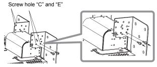
**5** Use no less than two commercially available screws (no less than four screws on both sides) for the screw holes  $(10-\phi8)$  on the stand bottom plate, to anchor the monitor. (Use screws having enough holding strength and resistance against external force of expected vibrations.)
