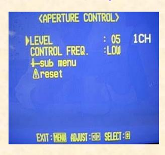
Compensates the frequency characteristics of the input video signal.
