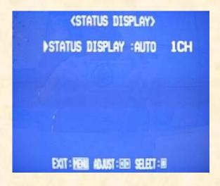
Sets the items related to the display screens, such as the status display or the AUDIO LEVEL METER display. Can also be used to set the 1080/60i or 1035/60i signal displayed correctly.
