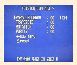
Compensates the picture distortion, tilt, and the color heterogeneity caused by the geomagnetic influence.
