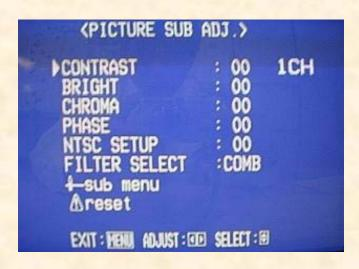
The standard value ("00") of the picture adjustment is initially set at the factory. You can adjust the standard value as your initial setting.
