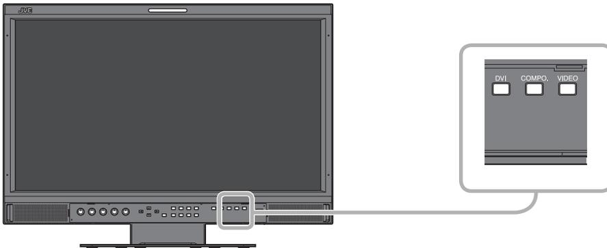
When the screen goes blank, and one or some of the INPUT SELECT lamps (DVI, COMPO., VIDEO) on the front control panel start flashing...
