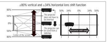
The vertical and horizontal lens shift function cannot be set to the maximum values simultaneously.
