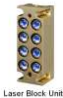
One of 6 banks of 8 Laser Diodes used in the DLA-RS4800
