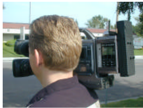
FireStore DR-DV5000 conveniently mounts between the camcorder and battery system on JVC GY-DV5000 series camcorder.
