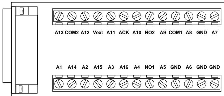
This drawing shows the Alarm I/O PCB supplied with the unit. This wiring interface greatly simplifies all alarm and VCR connections to the unit.
