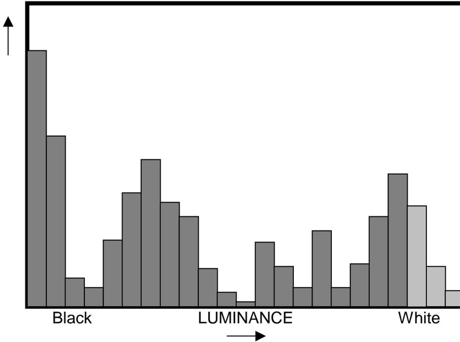
In Figure 1, the camera has a wide range of luminance, or Grey scales and shows a signal with a high level of detail. This signal will be suitable for video motion detection applications because high detail is present.
