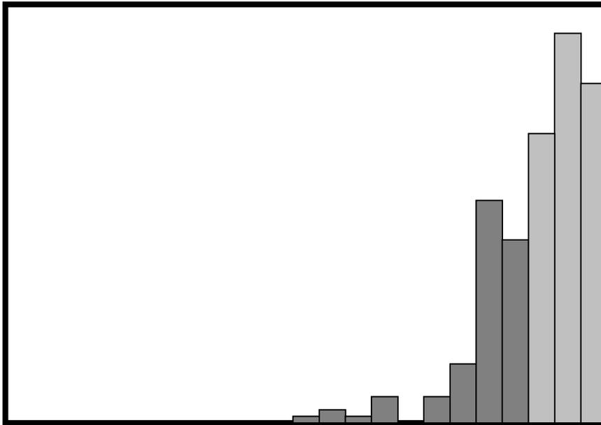
In Figure 3, the camera's lens or its AGC is out of adjustment, resulting in high luminance levels. As a result, detail in the scene is likely to be lost during multiplexed recording, and video motion detection will be ineffective.
