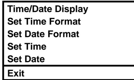
The time can be in one of two formats, and date can be in one of three formats. Time format can be either a 12-hour or 24 hour clock. Date format can be either DD/MM/YY, MM/DD/YY, or YY/MM/DD.
