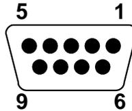
The figure shows the socket on the multiplexer as seen from the back of the unit. The numbers are marked on the connector itself, although they may be difficult to read.
