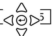
Pop-up menus are the last levels in the menu system. In general, use the left/right arrow keys to select sections in the Pop-up menu and then use the up/down arrow keys to make changes to the values. There are, however, some Pop-up menus where the arrow keys have additional functionality.
