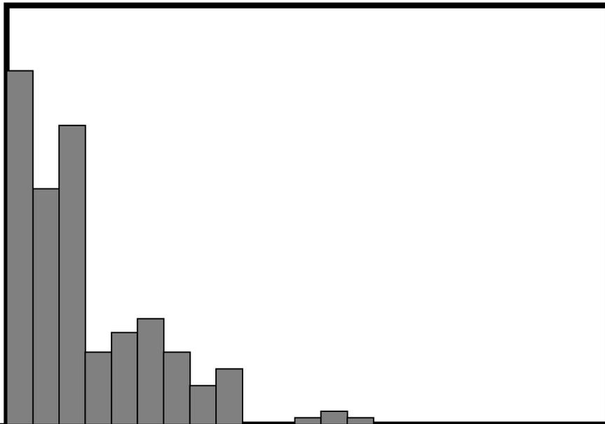
In Figure 2, the camera's luminance levels are low and have a smaller range, so that it will be more difficult for the user to see detail both when viewing live displays of the camera as well as when reviewing multiplexed recordings of the camera. This camera will also not be suitable for video motion detection, because relatively few Grey levels will be digitized and changes with time are less likely to be detected by the VMD circuits.
