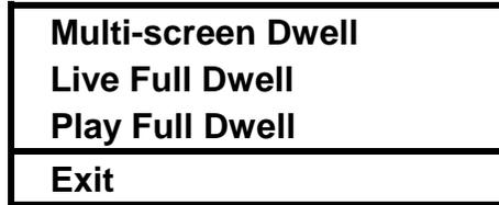
The full-screen dwell times are the same for both Monitor-A and Monitor-B in Live and Play modes. Dwell time settings determine the time between each camera sequence in the sequence list.
