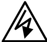
The lightning flash with the arrowhead symbol, within an equilateral triangle, is intended to alert the user to the presence of uninsulated "dangerous voltage" within the products enclosure that maybe of sufficient magnitude to constitute a risk of electric shock to persons.
