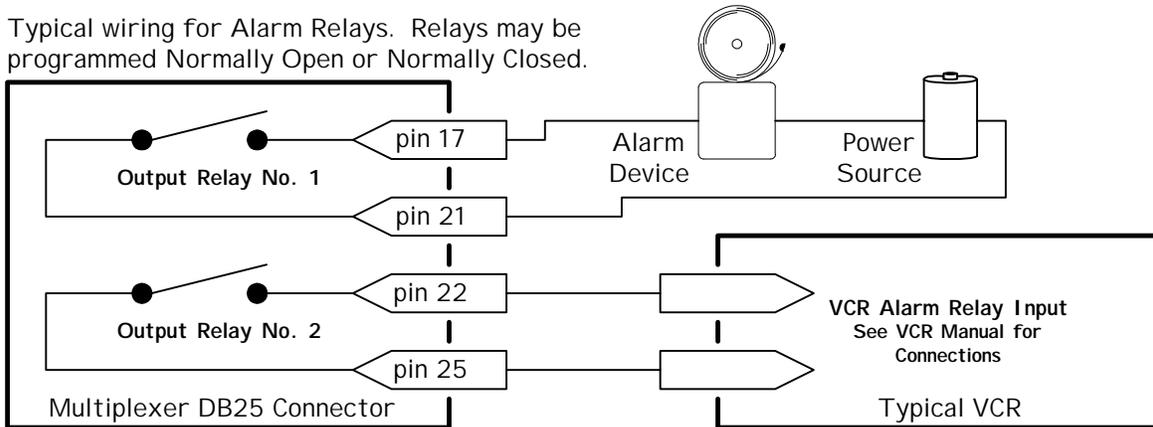
The alarm output relays can be programmed in the menu system to respond to macro functions, alarms and video loss. Connect your application to the alarm output relays (resistive loads only).
