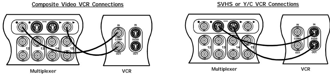
Refer to the specific instructions provided with your VCR and connect the multiplexer's Record output to the VIDEO IN connector on your VCR and the multiplexer's Play input to the VIDEO OUT connector on your VCR. The drawings above are illustrative of typical multiplexer to VCR connections.
