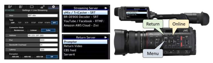
SRT protocol features real-time stream quality confirmation with the status displayed in the camera's LCD/EVF. When the receiver (decoder) detects the excessive data loss which cannot be corrected with the built-in error correction, the "LIVE" indicator will change color to notify the cameraman / talent that transmission quality may be compromised. Detailed stream quality data is available when pressing the "Status" button on the camera.
