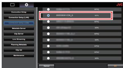
④ For configuring information required for connecting to a wireless LAN access point.
