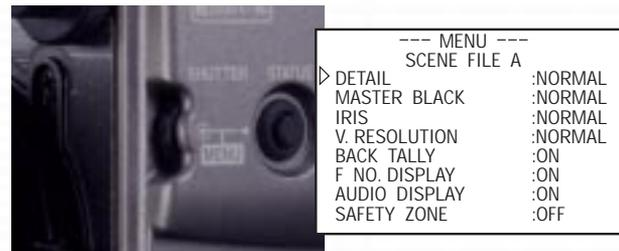
A built-in menu dial lets you quickly and easily navigate through the viewfinder menu, as well as set the shutter speed.
