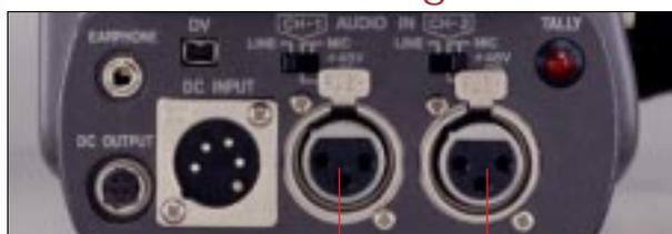
To complement its superior DV pictures, the GY-DV500U offers outstanding digital PCM sound. You can choose between two 16-bit 48-kHz channels or two 12-bit 32-kHz channels with a dynamic range of more than 85 dB.
