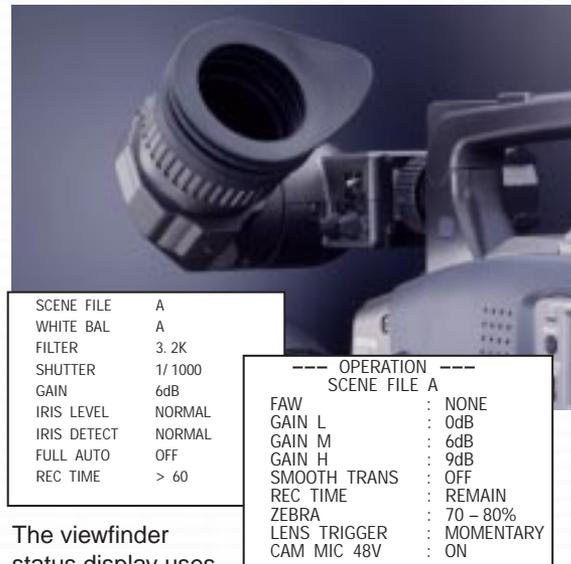
The viewfinder status display uses characters and menus to display selected information in the viewfinder, including various events, camera setting status, recorder operation, and selected setup parameters.
