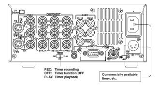
When power (AC 120 V (U MODEL), AC 220 - 240 V (E MODEL) or DC 12 V) is supplied to this unit, it automatically enters the Record or Play mode. Using a commercially available timer, you can configure your VCR to start recording or playback at a specified time
