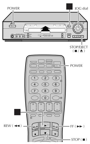
**To prohibit operations during playback (Mode Lock)** Press and hold **OK** on the Remote for more than 5 seconds. "→" and "→1" light up on the front display panel (() pg. 60). The playback will not be interrupted until the recording end (unrecorded portion) or tape end is reached (() pg. 37, 41).
