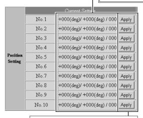
The current Pan/Tilt/Zoon position can be set to any of the 10 position memories by clicking on "Apply".
