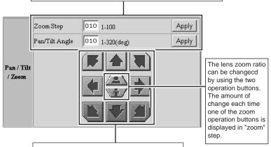
The Pan/Tilt can be controlled with the 8 Pan/Tilt operation buttons.
