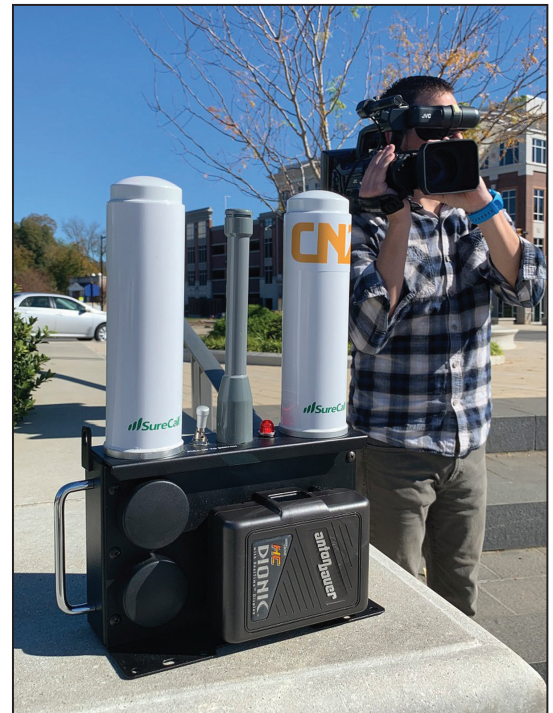
CN2's Rob Barnes demonstrates the cable station's new JVC ProHD Portable Bridge, which allows the cable station to stream live footage directly to its website or back to the station for live ENG reports for its daily newscast.
