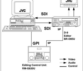
The BR-D85U can serve as source and recorder; while computer graphic software controls the BR-D85U and performs layering of graphic images.
