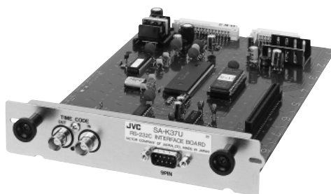
SA-K37U RS-232C Control I/F Board for BR-S522XU, BR-S622XU, BR-S822XU and BR-S800U, BR-S500U
