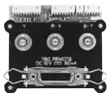
SA-K27UA RS-232C Remote Board for BR-S522U/DXU, BR-S622U/ DXU, BR-S822U/DXU, BR-S800U, BR-S500U and BR-S605UB
