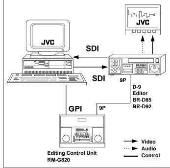
The BR-D85 can serve as source and recorder; while computer graphic software controls the BR-D85 and performs layering of graphic images.
