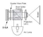
FIGURE 4: Optical Schematic of Basic D-ILA Projector
