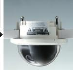
**4.** Mount the ceiling panel to complete installation.
