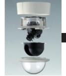
1. Remove the camera's outer cover and ceiling
