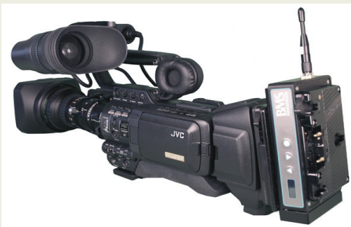
Fig. 8. JVC's ProHD ENG camcorder fitted with BMS 2GHz microwave camera-back unit (the LIBRE transmitter). The BMS camera-back accepts the compressed MPEG-2 TS (Transport Stream) of 19Mbps, modulates 16-QAM and transmits COFDM over 8MHz bandwidth for roving robustness in HD ENG, sports and EFP applications.
