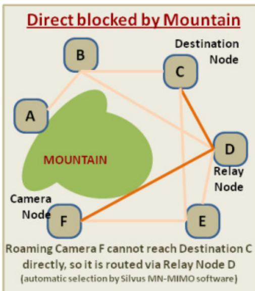
**Every MESH Node is a radio transceiver**, capable of transmitting, receiving, buffering, and forwarding data in UDP/TCP protocols over the IP-based private radio communications channel. The quantity of Nodes required to cover an event is of course subject to the size of the area, the local topography (is the area mountainous, hilly or relatively flat, or urban) and the extent of desired coverage. Buildings may impede connectivity, but also provide benefits in the form of RF reflections.
