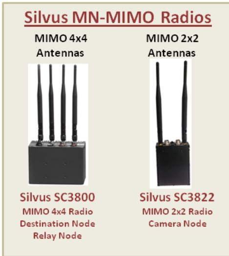
**The Camera Node** (generally a SC3822 Radio) – as a camera-back/side attachment, accepts a LIVE H.264 compressed IP encapsulated HD feed over the Camera’s USB host connection, seeing the Node (Radio) as a standard LAN connection. The MESH Network is indeed a LAN but a wireless one (WLAN). The Camera Node also provides for return audio and IFB connectivity. The Camera Node modulates the IP packetized HD video in COFDM in its RF transmitter section.
