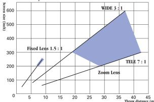
In the shaded areas in the graph, the projected image may be partially distorted or missed out depending on the distance between the projector and the screen. To project an image with no image distortion or missing, we recommend you to use the projector in the areas defined with solid lines in the graph.
