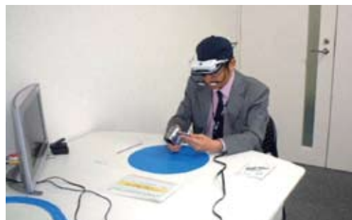
Scene of user test (operation test of video camera using eyemark recorder)
